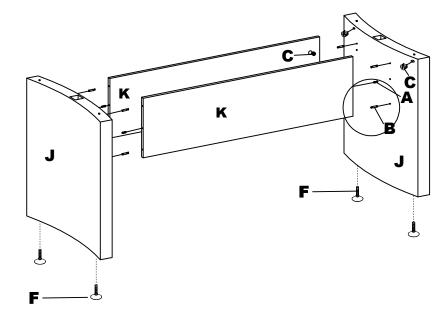
NOTE: The arrow on the face of the Cam (C) should point towards the Cam Post (B) for proper alignment.
