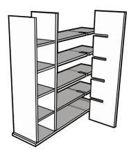
Step 8: Insert Top Shelf parallel to Bottom Shelf, fitting the grooves of the Top Shelf into remaining grooves of dividers. Make sure back grooves are aligned. Edge of shelf should be inserted into remaining mortise of Side A Panel. Insert hex screws into (2) pre-drilled holes in Side A Panel and tighten down halfway.
