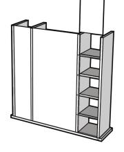
Step 12: Slide remaining Small Back Panel into the back grooves of Top Piece and the Top Shelf until the edge rests firmly in the back groove of Side A Panel.
