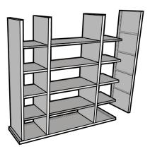
**Step 9:** Insert edge of Top Piece into remaining mortise of Side A Panel while aligning the back grooves. Insert edges of each divider into the corresponding mortise on Top Piece. Insert hex screws into (4) pre-drilled holes of the Top Piece and tighten down half way.
