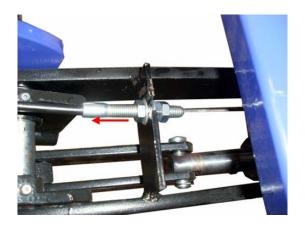
b) Loosen the up and down nuts, Pull the release wire down, and then tighten the nuts until the table lowers
