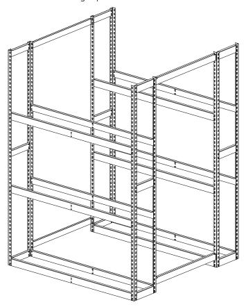
NOTE: Cross Aisle Ties are REQUIRED to be used for unit stability on Double Entry Units.
