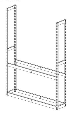
**8.** Place the final left-to-right channel supports near the top of the unit. Attach the shelf support in the center.
