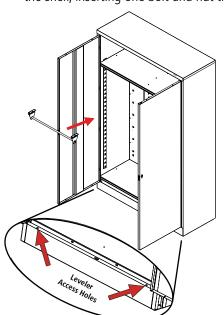
on the far right and far left side. The open side of the side brackets should face into the unit. Place the last bracket on the coat rod (Ref. No. 11) and insert the rod into the other by flexing the second bracket. Secure the bracket to the middle of the shelf with one bolt and nut through the hole provided in the center of the shelf. At this time. tighten all of the nuts and bolts around the entire unit.
