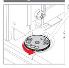
For best punch results, occasionally rotate the punch disc
