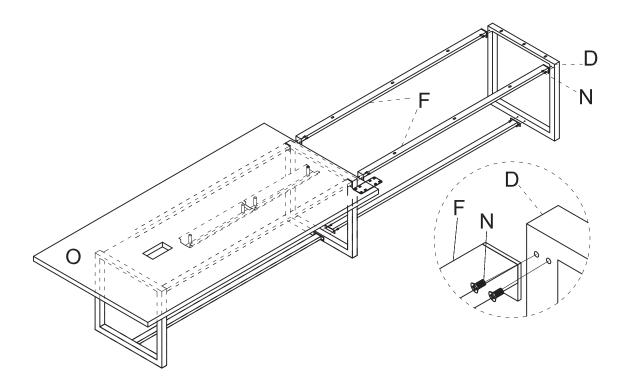
Use the Screw (M) to connect the Frame and the Top (O), Use the Screw (N) to install the Bracket (J) to the Top;
