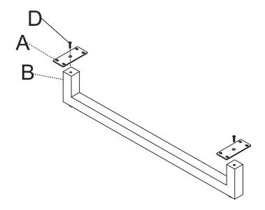
Use Screw (E) to connect the U Shape Base (B) and the Bracket (A) to the bottom of the Pedestal.
