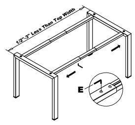
Place Top (Seperate Carton) upside down on a clean, flat surface. Attach Top Mounting Clips (D), Qty 4, to underside of top at pre-drilled hole locations using Screw (G) Qty 8.
