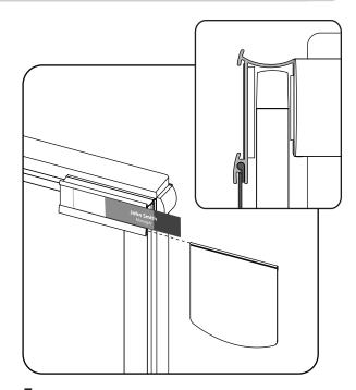
Slide dry erase board into bottom slot of nameplate. Print name/title on 7" W x 1.75" H sheet. Remove lens from nameplate. Insert printed name into nameplate and replace lens.
