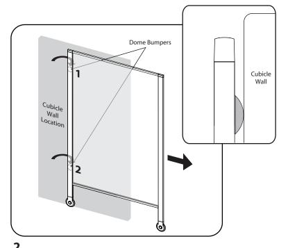
Remove protective film from back of (2) dome bumpers and apply to the inside of the rear leg (see image above 1, 2).
