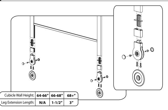
For cubicle panel systems 66" and taller, attach the recommended 1-1/2" or 3" leg extensions to the privacy screen according to the chart above. Use flat head screw driver to remove front and back wheel housing caps. Remove wheels and wheel housings. Insert extension connectors into screen leg uprights. Press 1-1/2" or 3" leg extensions into extension connectors. Replace wheel housings, wheels and wheel housing caps.
