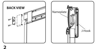
**Remove** track end cap on opposite end of screen mounting plate. Slide J-Hook into back channel of track. **Note:** bottom of J-Hook must engage channel in back of screen. Slide nameplate over front face of track. Replace track end cap.
