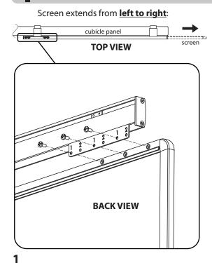
For installation with screen extending from <u>left to right</u>: Insert (3) #8-32 x 3/8" Pan Head Screws through holes marked "1" in mounting plate into threaded nuts in screen as shown above. Tighten firmly.
