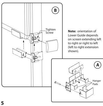
(A) Slide Lower Guide over Lower Hanger Bracket and insert (2) #10-32 x 1/4" screws through lower guide into hanger bracket. Tighten firmly. Follow steps in **3B** to attach the correct size Inner Hanger Bracket to the Lower Hanger Bracket and apply hanger pads as indicated. (B) Slide hanger bracket onto panel and position lower guide so it engages the screen but does not support it. Tighten the hanger bracket screw firmly. Press bracket cover into place.
