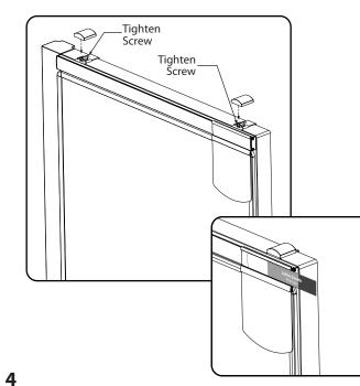
Slide hanger brackets over cubicle panel and tighten screws. Align bracket covers with hanger brackets and press into place. Print name/title on sheet and cut to 7'' W x 1.75'' H. Slide lens from nameplate. Place printed name behind lens. Slide lens and printed name back into nameplate.
