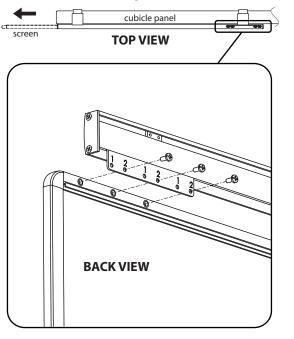
For installation with screen extending from **right to left**: Insert (3) #8-32 x 3/8" Pan Head Screws through holes marked "**2**" in mounting plate into threaded nuts in screen as shown above. Tighten firmly.
