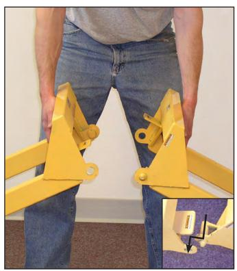
3) Bring the two halves together. Align and simultaneously insert the pins on each half into the corresponding holes on the other half.
