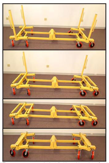
The support arms can be installed in a wide variety of positions depending on the support needs of the load being carried.
