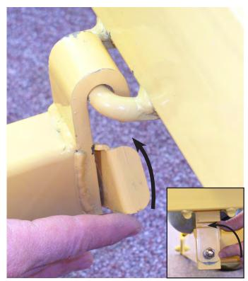
2) Close the Frame Catch. **CAUTION**: Never use the Troll® Bridge  $^{\text{TM}}$  modular cart system without closing these catches. If the catches are not closed the Troll® Bridge  $^{\text{TM}}$  may detach from the cart possibly resulting in property damage or bodily injury.
