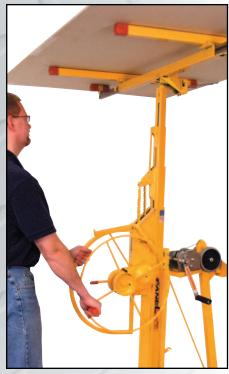
Install the board as normal using your PANELLIFT® Drywall Lift.
