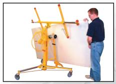
To load, lift board by one end and place in the foot bracket making sure it is centered on the bracket.
