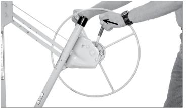
3. To lower the PANELLIFT<sup>®</sup> Drywall Lift control the backward rotation of the winch by grasping the winch handle with your right hand BEFORE releasing the brake with your left hand. ALWAYS use this two hand method when lowering the PANELLIFT<sup>®</sup> Drywall Lift.
