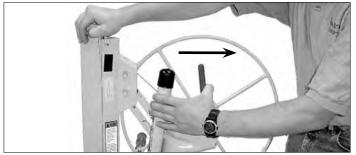
5. Place your right hand on top of the frame and pull the winch assembly towards you. While pulling the winch towards you, grip the brake arm sufficiently to prevent back-lash of the cable on the winch.
