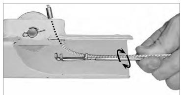
6b. With a clock-wise motion like that of tightening a screw driver, twist the cable installation tool while holding the crimped end of the cable up into the sheave pocket. The cable will pop loose from the tool and pop up through the sheave pocket as shown in this cut away view.
