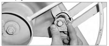
7. Now push the winch assembly back towards the frame. This action will automatically engage the slide bar lock. ALWAYS check to make sure that the slide bar lock is fully engaged by rotating it clockwise as far as possible before proceeding. The illustration shows a fully engaged slide bar lock. NOTE: DO NOT tighten the slide bar lock nut assembly. This will make it impossible to collapse the PANELLIFT<sup>®</sup> properly for transport and storage.
