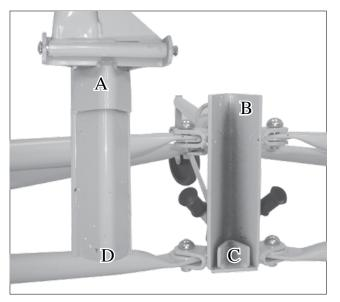
2b. Pocket "A" slides OVER angle "B" while angle "C" slides INSIDE angle "D".
