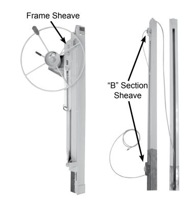
Inspect and replace sheaves (pulleys) before replacing the cable. There are 3 sheaves on the 138-2 Panellift<sup>®</sup>, one on the frame and two on the "B" telescoping section. Sheaves should be solid on their axle and not move up and down or back and forth. To replace, remove cotter keys and discard old axle and sheave. Replace with new sheave, axle and new cotter keys.
