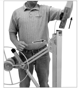
3. Remove the two telescoping sections completely from the frame housing. Pull the cable completely out from the frame along with them. BE CAREFUL for loose strands or frays on the cable.
