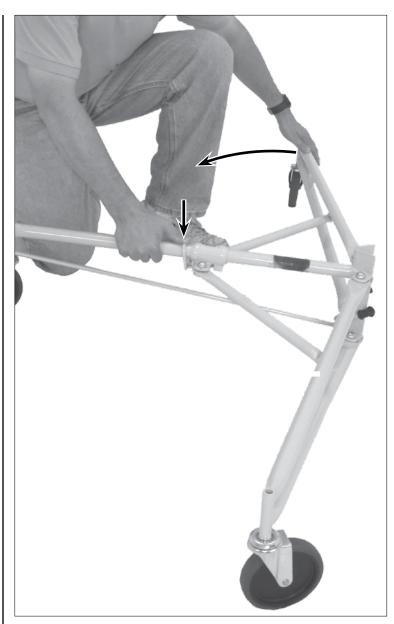
10. To collapse the tripod base, press down on the slide yoke pin clip and swing the legs in until they lock in the closed position.
