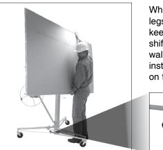
When the backstop legs are set, they keep the unit from shifting while loading wallboard or while installing the frame on the tripod base.
