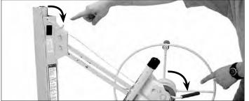
6. When the winch is fully extended, release the brake arm and swing the retaining hook away from the telescoping sections.
