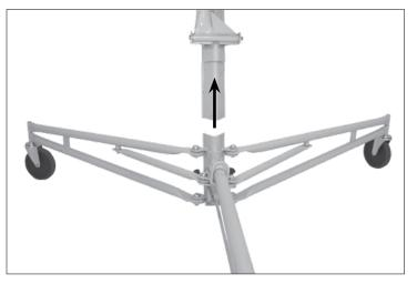
9. Lift the frame off of the tripod base.
