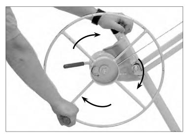
4. Rotate the winch forward one full rotation.
