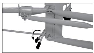
2c. To hold the tripod base in position during this procedure set the backstop as shown.
