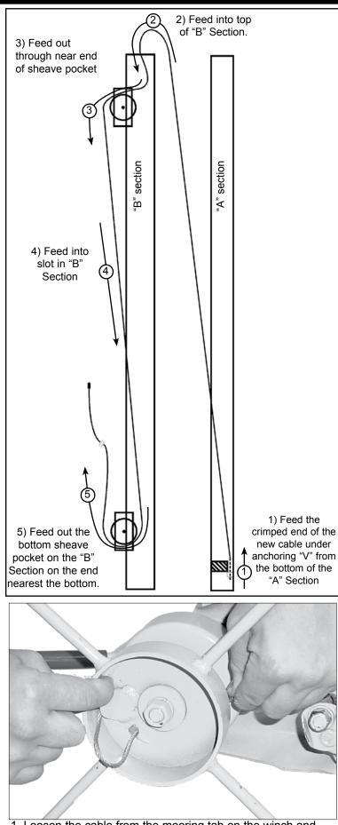
1. Loosen the cable from the mooring tab on the winch and pull it out from the winch drum. BE CAREFUL! A worn cable can have frayed strands. Wearing gloves will help protect your hands.
