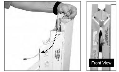
10. To reinstall the assembled telescoping sections, feed the crimped end of the cable through the frame sheave pocket from the top and over the top of the sheave as shown.
