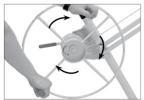
2. To raise the PANELLIFT<sup>®</sup> Drywall Lift rotate the winch wheel in the direction shown. The brake arm is spring loaded to hold the winch automatically at any height.
