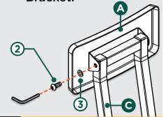
**Double check all** bolts to be tightened securely before use. **Check all screws** periodically. Failure to completely tighten the screws may result in tipping and possible injury!
