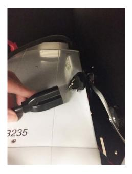
**2.** Plug the power strip into the inverter/charger.
