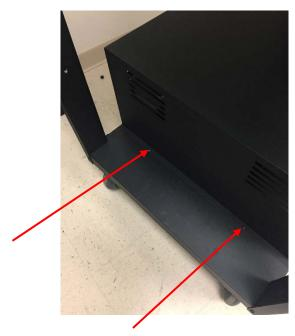
**3.** Reapply the (4) screws to sides of the battery box with supplied Allen wrench.
