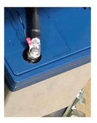
**9. Negative Connection, Battery 2:** Take bolt and place flat washer, small black wire (E), and black connector wire (D2) onto bolt (as shown above).
