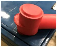
**8.** Securely tighten terminal bolts on Battery #1 with a 10mm wrench and pull rubber boot over tightened terminal.
