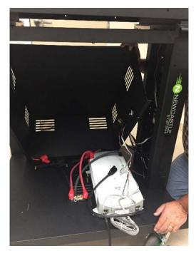
**5.** Carefully lift the battery box and make sure cables stay positioned through the plastic wire grommet.
