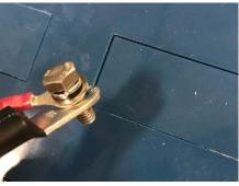
**6. Negative Connection:** Place lock washer onto bolt first, then flat washer, then small black wire (C), then large black wire (B) in order shown above.
