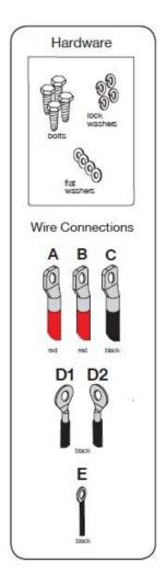
Wire A (red) connects to red positive (+) battery terminal of Battery #1.
