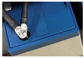
6. Negative Connection, Battery 1: Take bolt and place flat washer, black connector wire (D1) and large black wire (C) onto bolt (as shown above); insert into negative (-) battery terminal.
