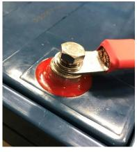
**4.** Securely tighten terminal bolts on Battery #1 with a 10mm wrench.
