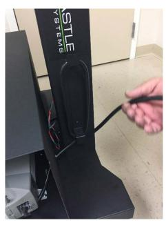
**3.** Run charger cord through cable opening and securely wrap around cord reel holder.
