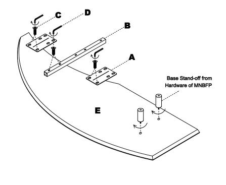
2 Attach Mntg Plates (A) and Support Bar (B) to the underside of adjacent Main Desk using Screws (C) and Wrench (D). Install the Top of MNRTNL to the underside of MNBFP using Screws and Base Stand-off.
