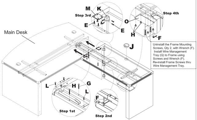
**5** Install Wire Management Tray (Q) to Frame using Screws (H) and Wrench (F).
