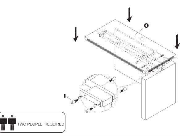
Unscrew the Screw, Slide the Adjustable Cross Bar (O) to suitable position, Use the Screw (G), (L), (H) to attach the Adjustable Cross Bar (O). Tighten the Screw back. Use Screw (E) and Corner Bracket (K) to attach the Fixed Modesty Panel (P) and the Leg of the Main Desk Put the Grommets (J) to the Top (O). Use Screw (E) and Plate (M) to attach the Top (O) and the Top of the Main Desk
