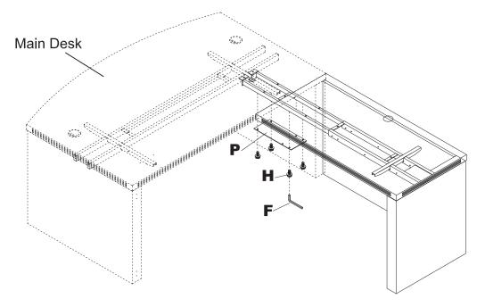
NOTE: Before assembly the top to metal frame, adjust the **SAME HEIGHT** of both **wood legs**
