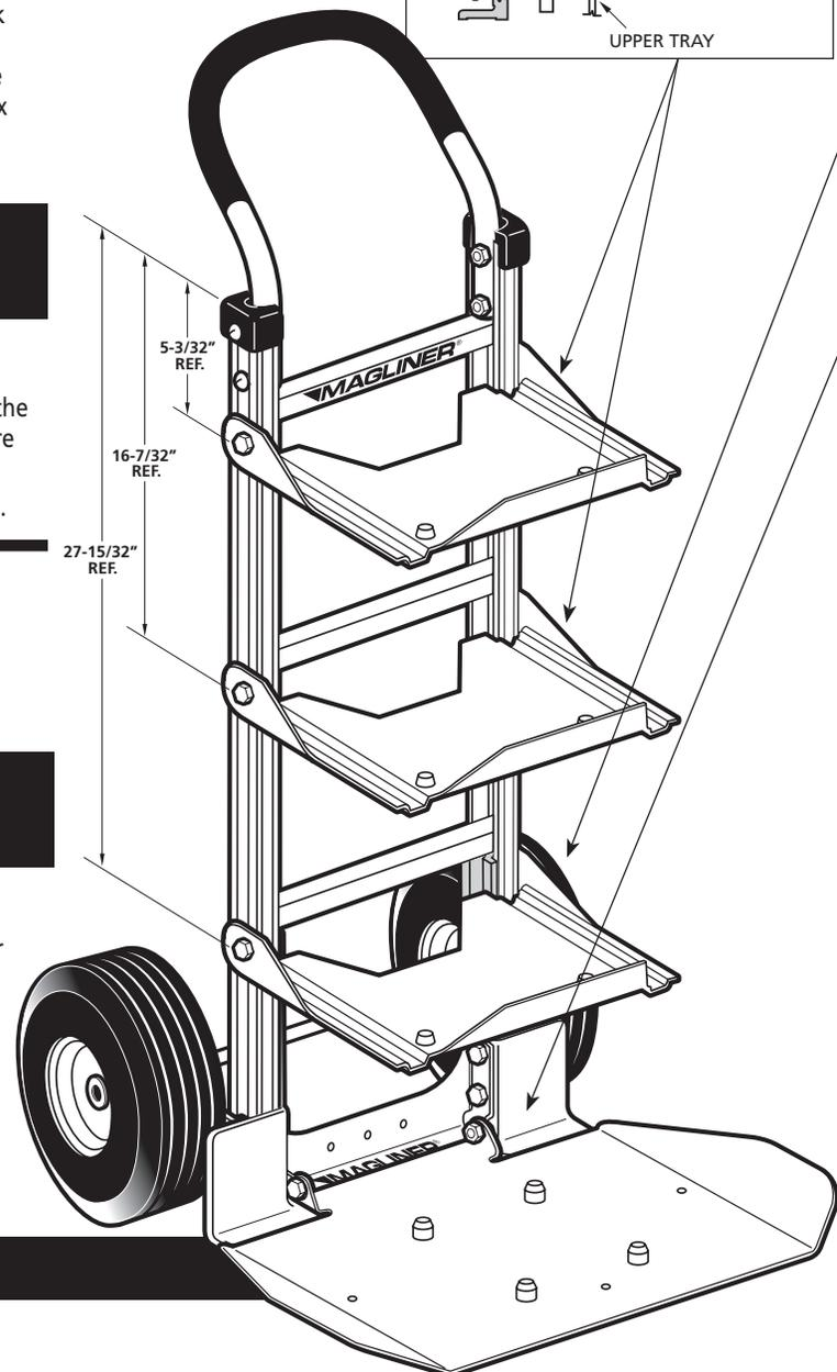
The hex bolts and nuts attaching the folding trays should be adjusted to hold the trays in the vertical position when not being used, and still allow the trays to be moved to the horizontal position. **Periodic adjustment may be necessary.**
