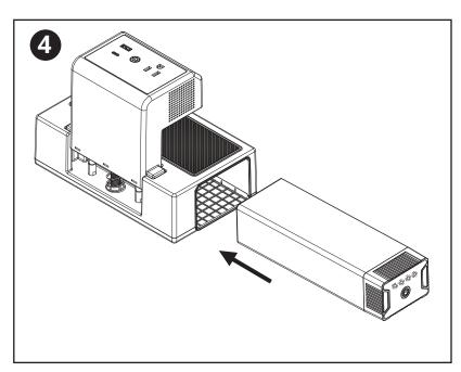
Insert Rechargeable Battery into Clamp-On Desktop Charging Unit. IMPORTANT: Battery must be fully charged before first use.
