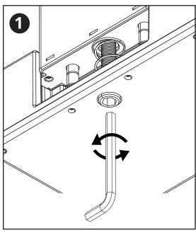
Open Clamp-On Desktop Charging Unit clamp by loosening 8 mm bolt.
