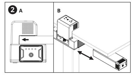
Test clamp fit by sliding clamp over edge of desk or table.
