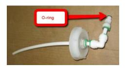
3. Check each tubing connection from the fresh water tank to the pump to make sure they are pushed together tightly. If the connections are not tight together, the pump will be pulling in air and won't be able to pump water.
