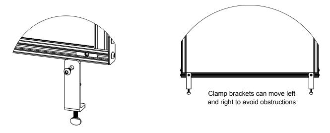
**Step 3:** Tighten thumb screws to secure panel to table top.
