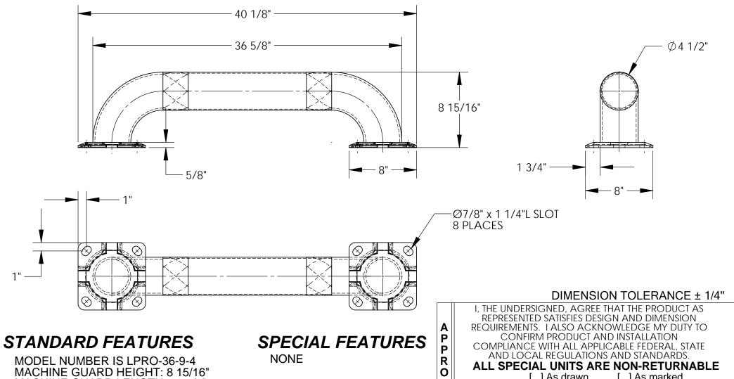
MACHINE GUARD LENGTH: 36 5/8" MACHINE GUARD DIAMETER: Ø4 1/2" OVERALL LENGTH IS: 40 1/8" **INCLUDES 2 MOUNTING BRACKETS** YELLOW POWDERCOAT FINISH **BLACK & YELLOW SAFETY TAPE** ALL STEEL CONSTRUCTION (ASTM A-36 MIN.) WITH **WELDINGTO MEÉT AWS** WARNING: CHECK APPLICABLE STATE & LOCAL LAWS FOR YOUR AREA
