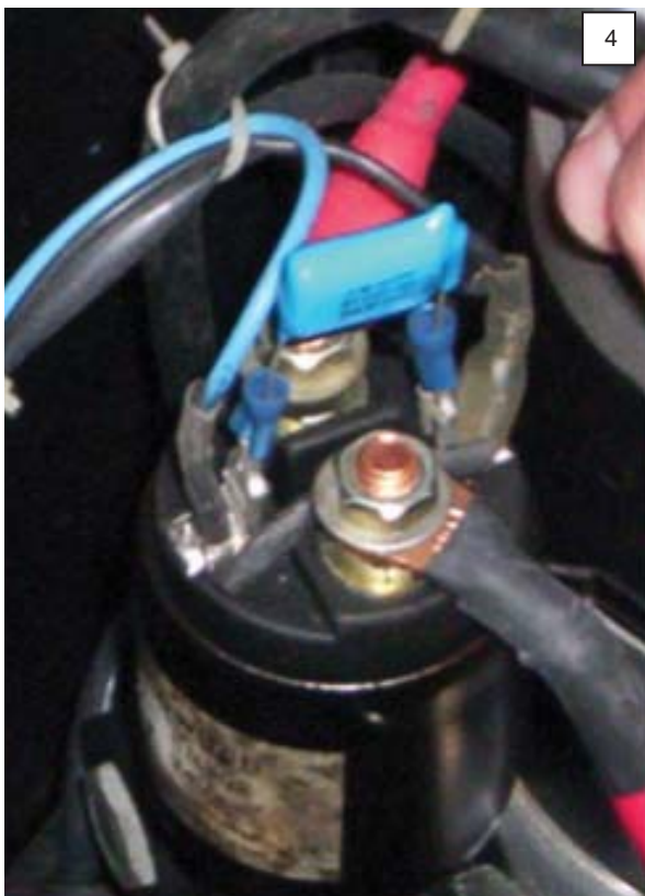
Quencharc installed on pump solenoid.
