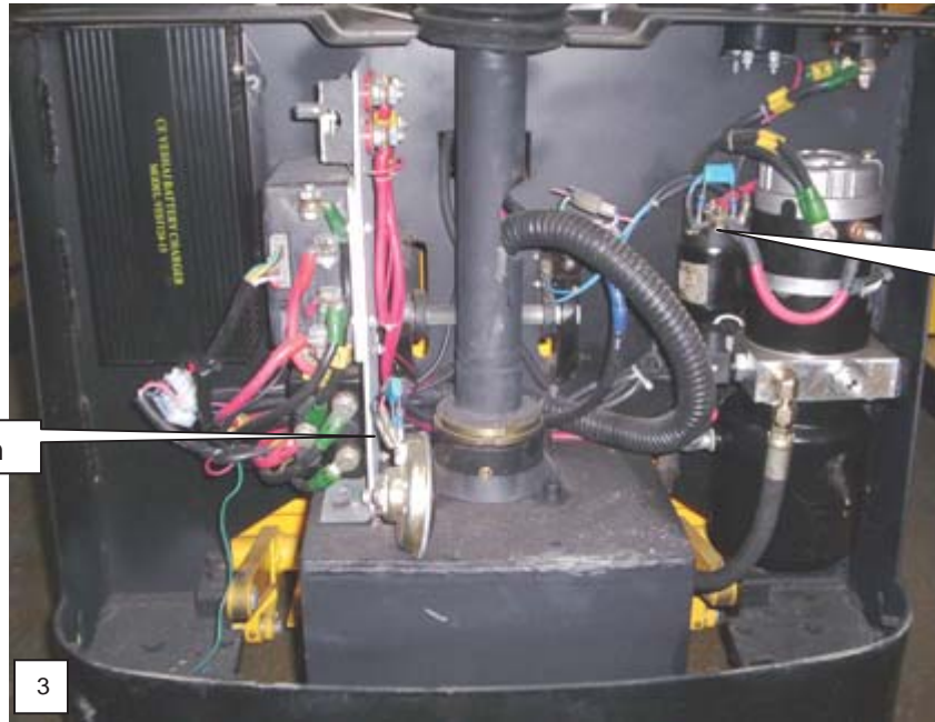
Quencharc installed on pump solenoid.
