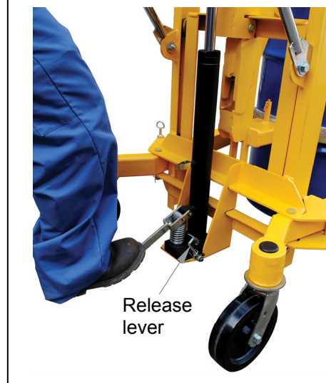
Press foot pump treadle to raise carriage
