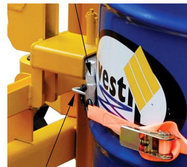
Attach strap hooks to drum saddle.
