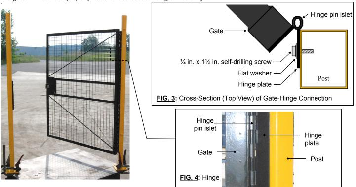
Use a 3/16 in. bit to drill holes for the self-drilling screws.
