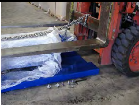
3. Attached the chain or steel cable on a fork lift. Get five M5X25 screws ready from the tool box.
