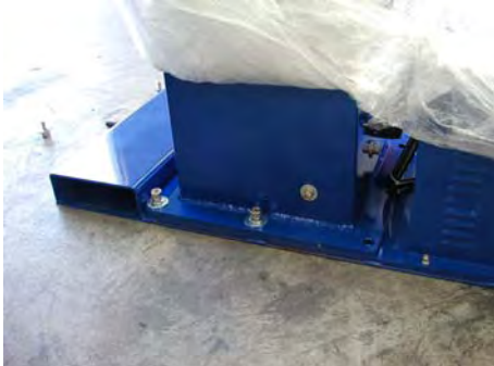
7. Use 5 M 12x25 Socket head screws with washers to tight up the Pillar on the base. Be sure those 5 screws have been fastened securely.
