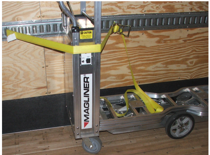
Figure 2: CooLift strapped into truck for transport
