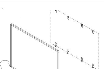
5 Secure top Angle Brackets (A) to the wall using long screws (B) as shown. Follow diagram in Step 1. Set board on the bottom angle brackets.
