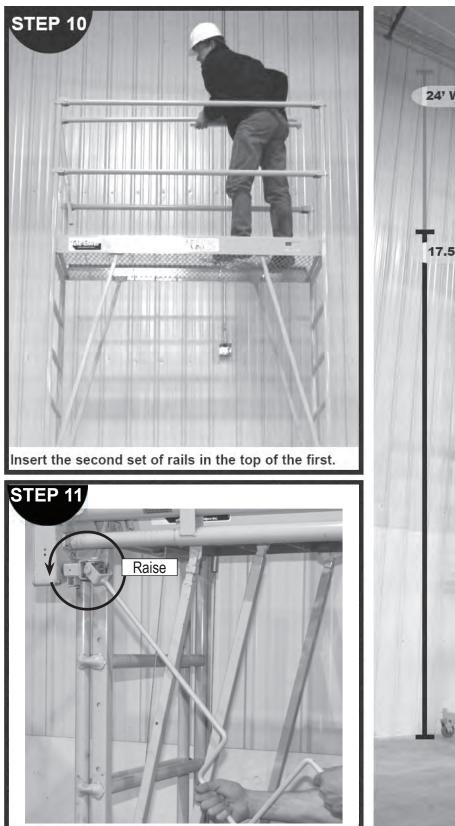
Raise deck to desired height by rotating winch handle in a counter-clockwise direction.
