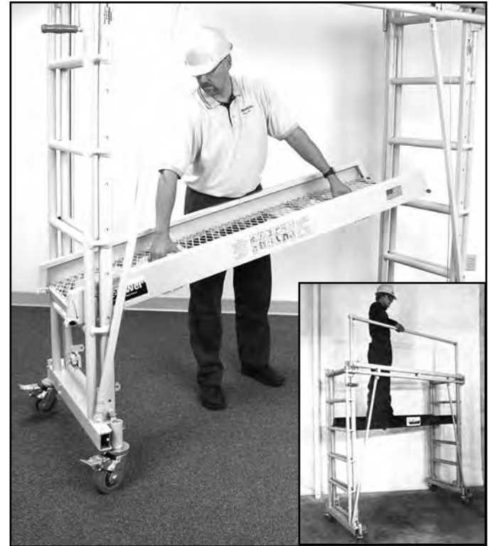
8) For platform heights from 2' to 6', the deck may be placed on lower rungs. For added safety use guard rails even when deck is on lower rungs.
